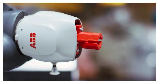
3D printed end-of-arm parts are more cost and time efficient than metal, with no reduction in capabilities
