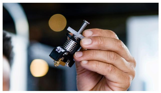
The print core CC Red has a wear-resistant ruby cone for printing abrasive composites
