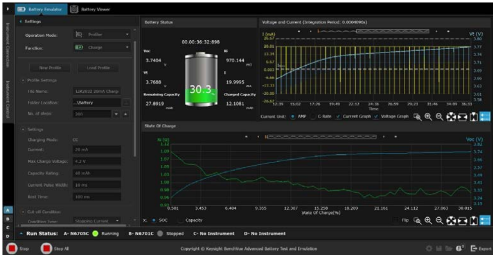
Figure 4. BV9210B creating a battery model
