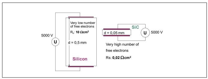
Figure 3 Dimensioning of 5 kV power devices – difference between silicon and SiC
