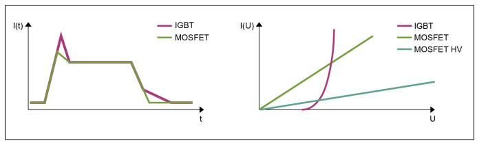
Figure 1 Comparison of the switching process (left, assuming same dv/dt) and the static I-V behavior (right) between MOSFETs (HV indicates a similar blocking voltage as an IGBT – 1200 V and higher) and IGBTs
