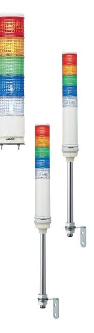
The Schneider Electric line of Harmony<sup>™</sup> XVC Tower Lights offers pre-wired, one-piece construction with five color combinations and integrated buzzer options in 40mm, 60mm and 100mm diameters. The entire XVC range meets IP54 (NEMA 12 and 3R) degree of protection.
