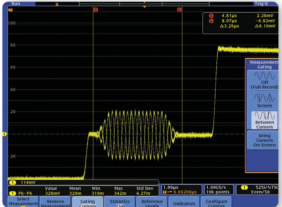
▶ Figure 10. An example of amplitude measurements on an NTSC signal. The peak-to-peak amplitude of the color burst is measured with the oscilloscope's peak-to-peak measurement. The area of the waveform the measurement is being taken on is gated by the cursors.
