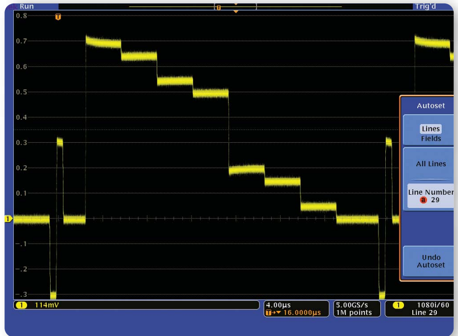
► Figure 7. The 4000 Series' Autoset feature makes setting up the oscilloscope for video as simple as a single button press.
