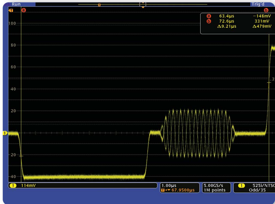
► Figure 12. Measuring the horizontal blanking interval from sync to start of active video on an NTSC color bar signal.
