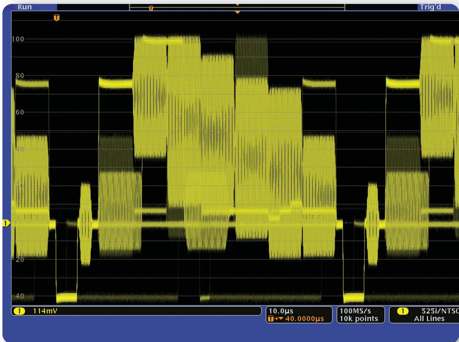
► Figure 9. A familiar video line rate display of signal amplitude vs. time on a digital phosphor oscilloscope illustrating the waveform monitor-like appearance of its intensity-graded display.
