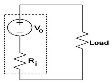
Figure 8. Circuit Model of Battery and Internal Resistance
