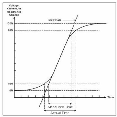
Figure 10. Slew Rate Measurement Graph
