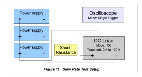
Figure 11. Connect the BNC to binding post adapter into a B&K Precision's 2542 oscilloscope. Follow the setup below for the DC load and oscilloscope.
