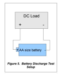
to idealize the internal losses in the battery when current is flowing. If the battery's electrochemistry is regarded as a network of voltage sources and resistances, then  $V_{\circ}$  and  $R_{i}$  comprise the Thevenin equivalent circuit. For alkaline batteries, the internal resistance goes up as
