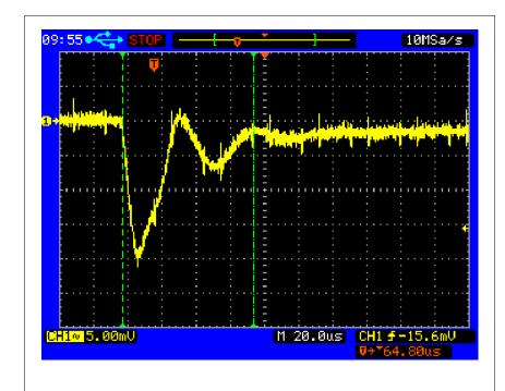
Figure 2. Transient Response for B&K Precision 9130
