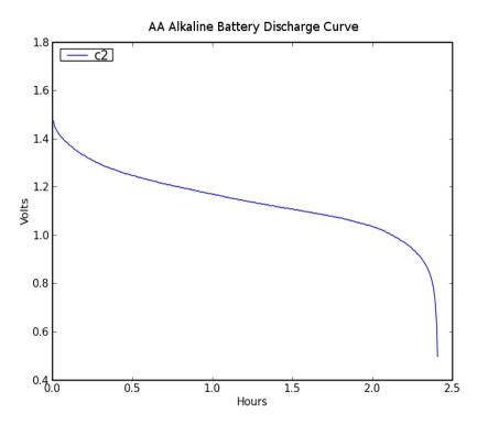
Figure 6. AA Alkaline Battery Discharge Curve
